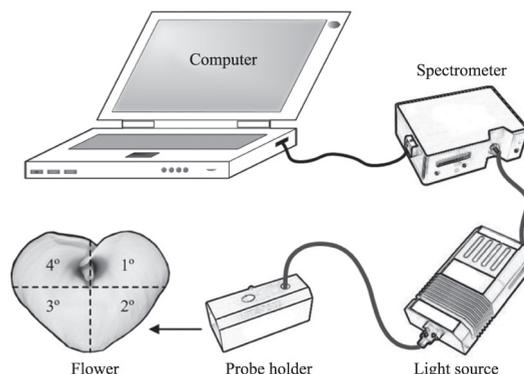
**Figure 2.** Scheme of the equipment used for measuring the spectral reflectance of calla lily flowers.
